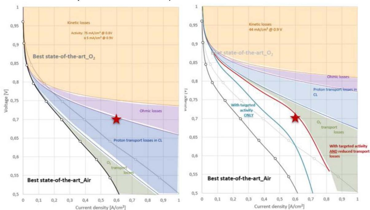
**Figure 1.** (Left) Performance with decomposition of the contribution of the different losses of the best State-of-the-Art (SoA) non-PGM catalyst with O<sub>2</sub> and Air vs PEGASUS objectives and (Right) PEGASUS non-PGM catalyst with targeted activity in Air: (blue) ~100 μm thick SoA non-PGM CL and (red) with reduced transport losses in ~50 μm thick CL. 80°C, 100%HR.
